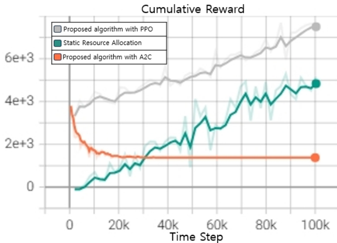
Fig. 4. Cumulative Reward, The performance of proposed algorithms using different methods in terms of cumulative rewards. The figure shows the performance of a proposed algorithm trained with PPO, a proposed algorithm trained with A2C, and a static resource allocation algorithm that consistently rewards only high quality. The experimental results show that the proposed method improves QoE by 55.01% compared to the method that does not consider data usage and by 444.21% compared to the static resource allocation method, providing users with a superior streaming experience.
